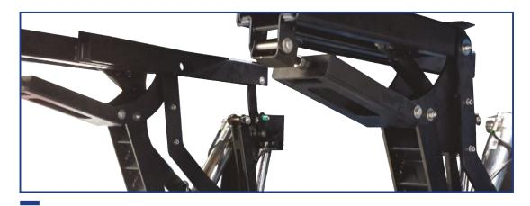
Thanks to the lift safety system, the platform is in-built with the deck when hooks are locked.
